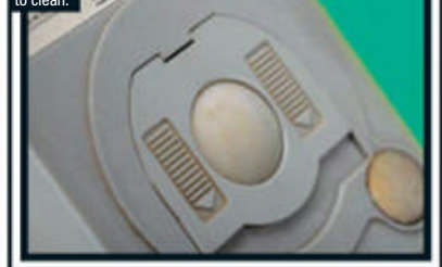
» The biggest problem with ball mice was that they would gather lots of dirt, thankfully they were easy to clean.
